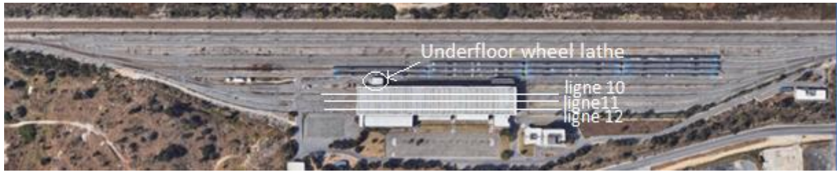
Figure 6 : Plane view of Fertagus maintenance yard
